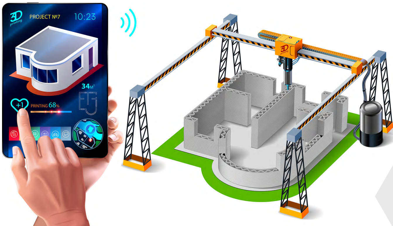
Figure 8 (3D Printing by extrusion and additive layers)
