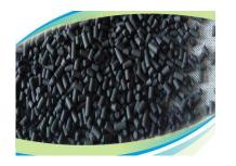
Carbon **Molecular Sieve** used in the **PSA Nitrogen** generation, the **Nitrogen** generation by Pressure Swing Adsorption (**PSA**) process is a technology used to separate **nitrogen** from a mixture of gases under pressure according to the special selective adsorption characteristics of the Carbon **Molecular Sieves** (CMS).
