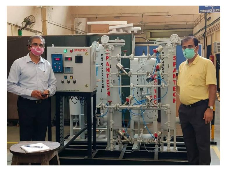
PSA Nitrogen Plant conversion to PSA Oxygen Plant
