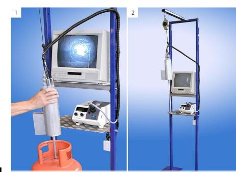
Equipment for internal inspection of LPG cylinders
