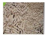
**PSA plant** employs **Zeolite** molecular sieves to separate the **oxygen** from the air. **Oxygen** with high purity is delivered whereas the nitrogen adsorbed by the molecular sieves is sent back into the air through the exhaust pipe. Pressure swing adsorption (**PSA**) process comprises of two vessels filled with molecular sieves and activated alumina.
