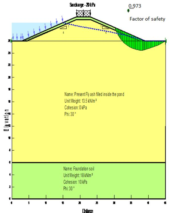
Figure 12: Output model showing Divider bund- Stability of Downstream slope- One side filled steady seepage condition
