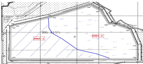
Figure 3. Plan showing demarcation of Area1 and Area 2 for raisings of ash pond
