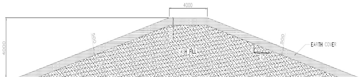
Figure 14. Typical cross-section of partition bund
