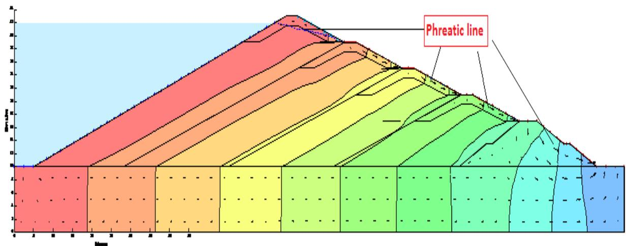
Figure 7: Output model showing Phreatic line from steady seepage condition
