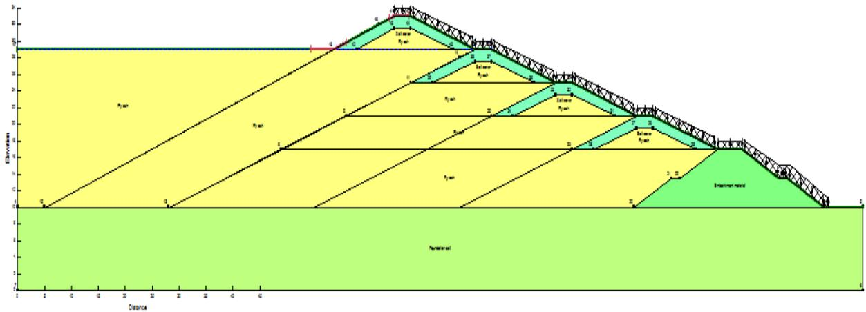
Figure 6: Input model showing 4<sup>th</sup> stage raising of ash pond
