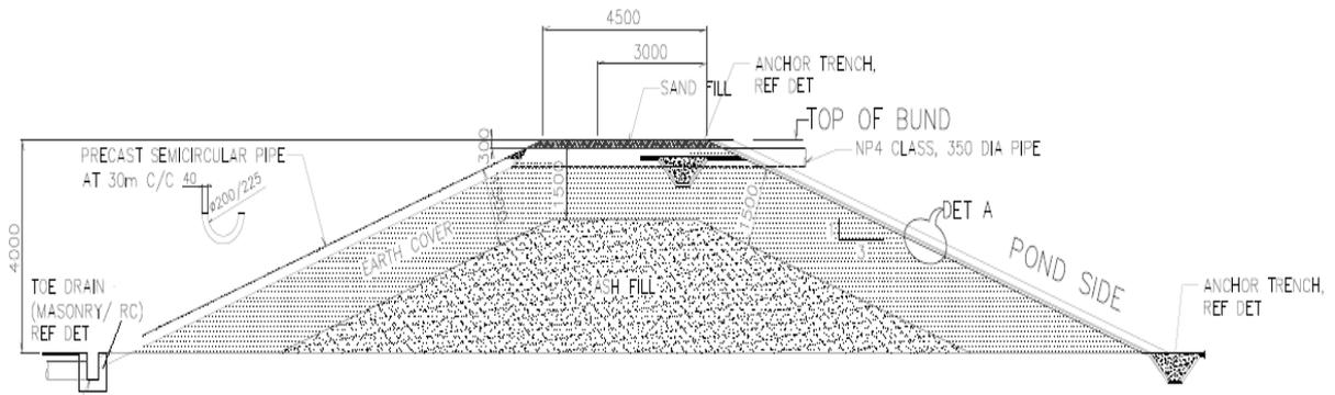
Figure 13. Typical cross-section of Peripheral bund
