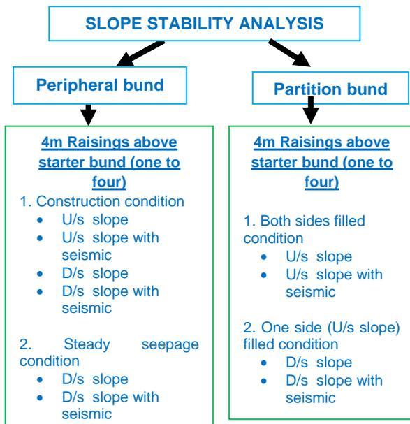
Figure 4. Flow chart of iterations of Slope stability analyses
