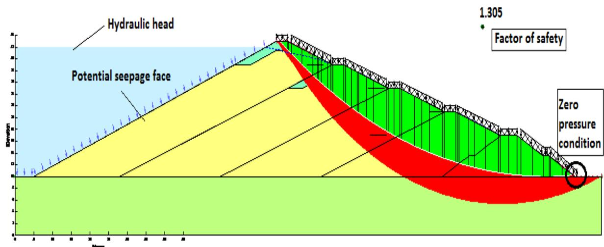
Figure 8: Output model showing steady seepage condition- With Earthquake forces
