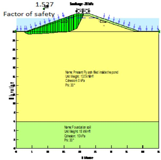
Figure 11: Output model showing partition bund- Stability of Upstream slope- Both side filled condition
