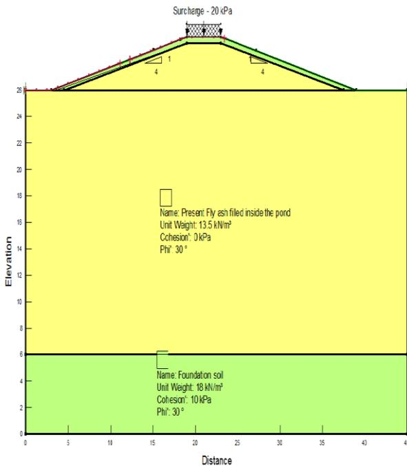
Figure 10: Input model showing partition bund at 4<sup>th</sup> stage
