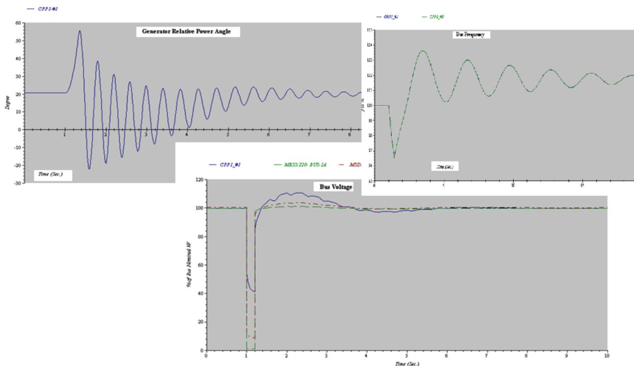
Frequency, Rotor Angle & Voltage Response of System following Grid Islanding and Load shedding
