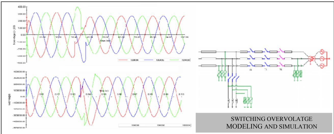
The voltage wave forms generated by the computer programme clearly show the over voltages at select locations and establish whether additional protection needs to be provided. They also show the effectiveness of such protection.
