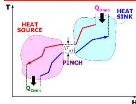
composite curve can be developed with vertical axis as temperature and horizontal axis as enthalpy (refer figure 1). These curves help the process experts to visualize the possible areas of improvements and implement the right solutions.
