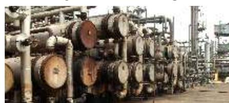
regards them as two flows with common energy content, one composite cold streams and one composite hot streams. The location where temperature difference ( $\Delta T$ ) for heat exchange between hot and cold stream is minimum is called pinch point.
