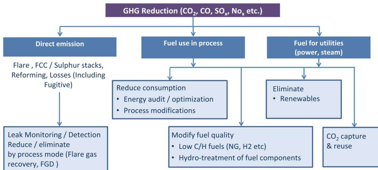
*Figure 1: GHG reduction: Source and control methods*
