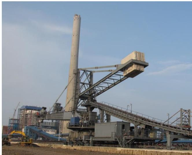
Fig -1 Stacker reclaimer equipment
