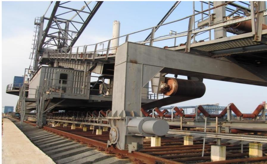
Fig – 5 Stacker reclaimer supported on flexible foundation
