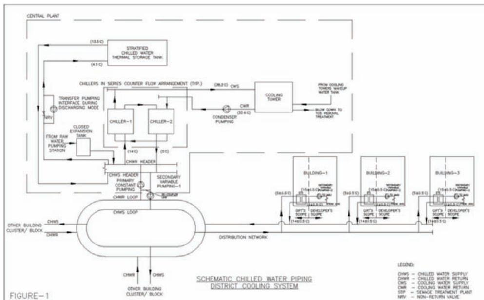
Figure 3: Overall schematic of a District Cooling System [7]
