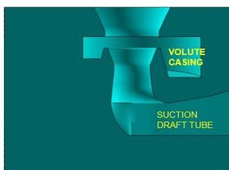
Figure-2 Sectional View through pump
