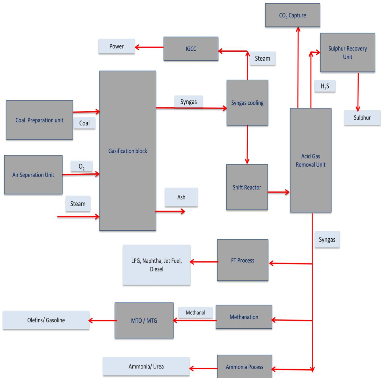
Figure 2: Block diagram of a typical CTL plant.
