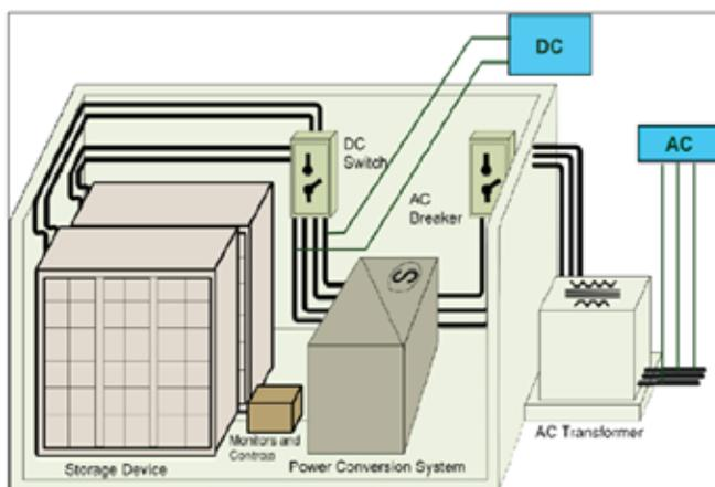
Figure 1: Schematic of Battery Energy Storage System
