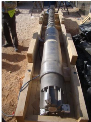
Well Head Pump 252m 3 /Hr, 297MWH, 3.3KV, 290KW Ready for installation
