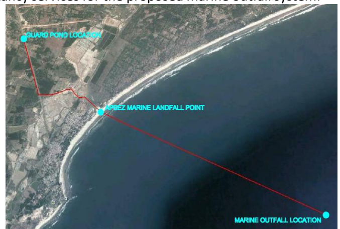
Alignment of marine outfall pipeline
